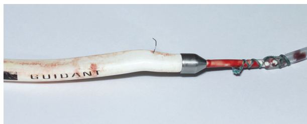
Fig. 1. Part of the flexible probe component protruding through the probe fascial covering.
