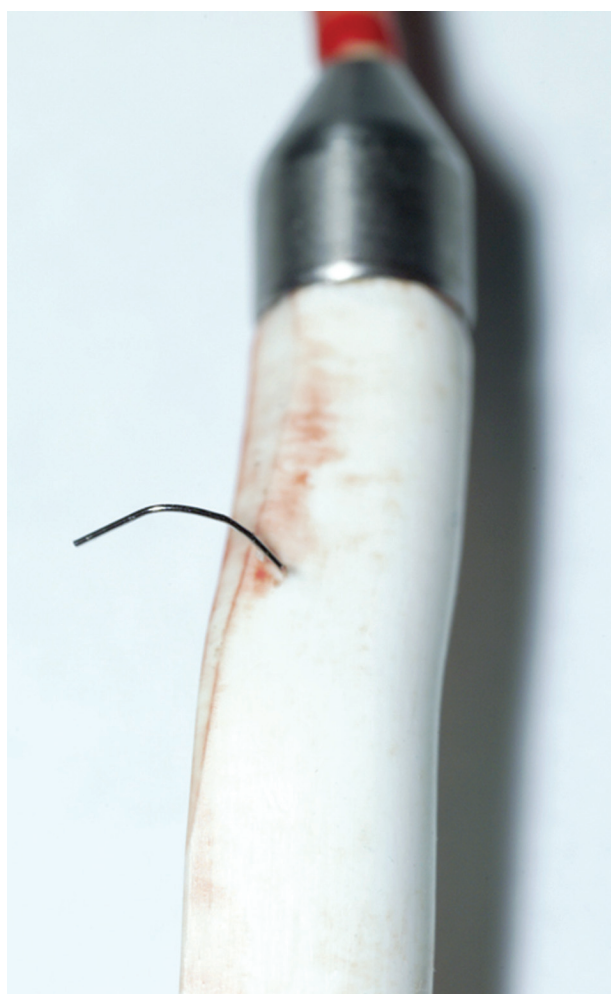
Fig. 2. Another view of the flexible probe component protruding through the probe fascial covering.
